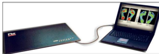
Fig 1: Shows the foot scanner device with computer connection
